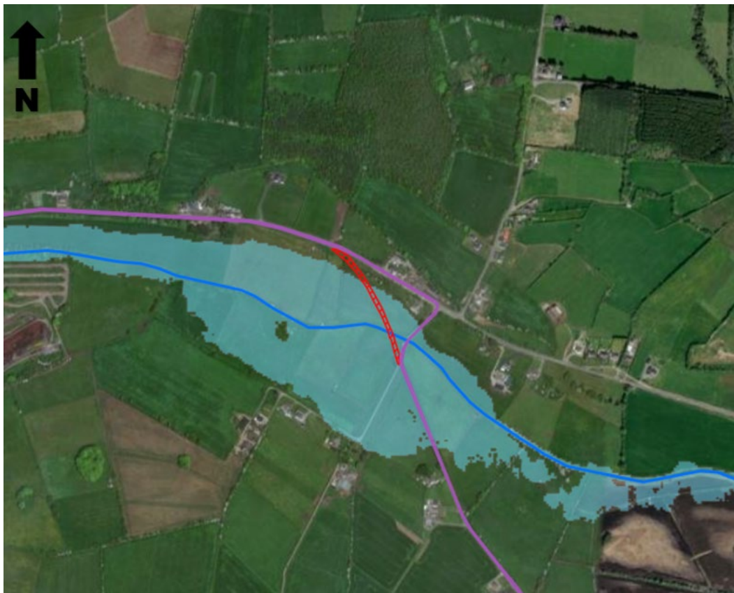
Figure 5-2: CFRAM Flood Map -Medium Probability-TDR Watercourse Crossing (Map from www.floodmaps.ie )
